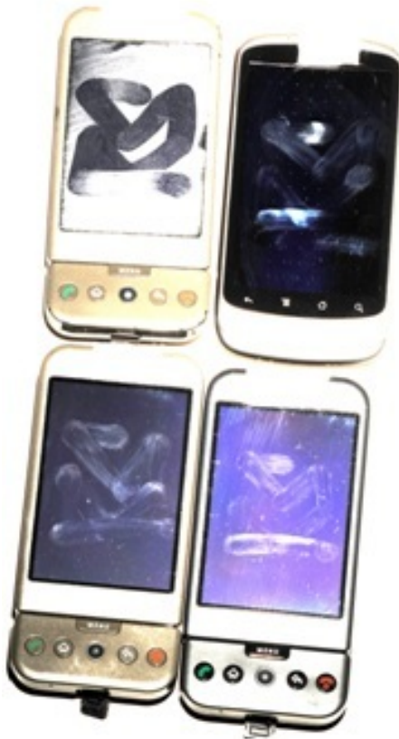
Figure 3.7: An image from Experiment 1: All four phones clearly displayed the pattern without the need to adjust contrast. Even the lightly touched Phone B ( lower-right ) has a visible pattern.
