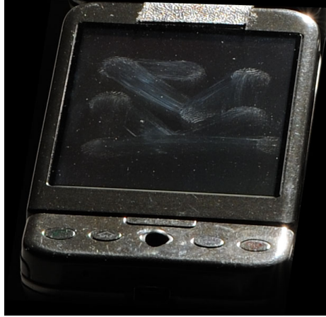
Figure 3.10: Phone A, from Experiment 1, where the pattern is entered with normal touches. Notice that the directionality of the pattern can be determined at every direction change.
