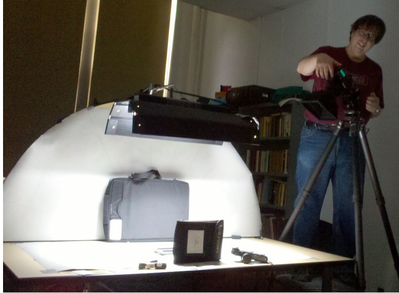
Figure 3.3: Photographic setup in practice: Matt Blaze taking a photo using a diffuse/soft light source at a angle of 90 degrees and a camera angled at 60 degrees.
